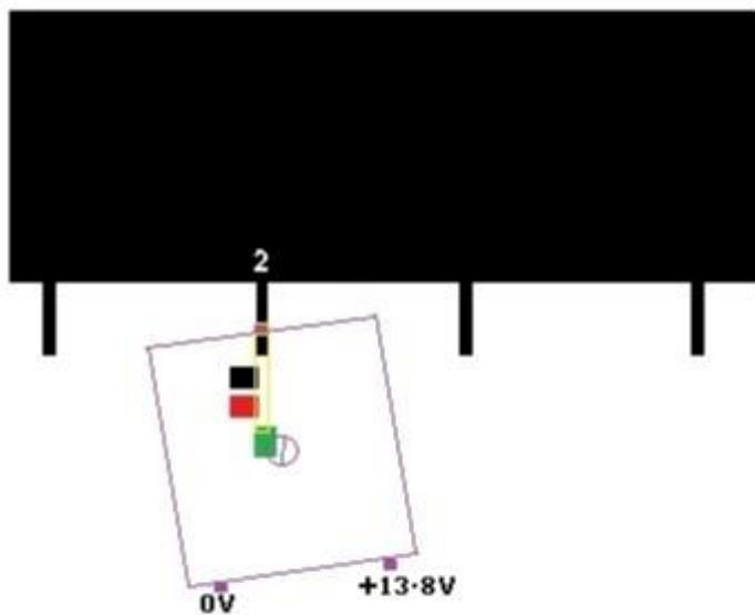
I found the best type of pot to fit is a square Iskra preset 10k ohms as pictured below – they have long enough pins to give clearance for soldering.
